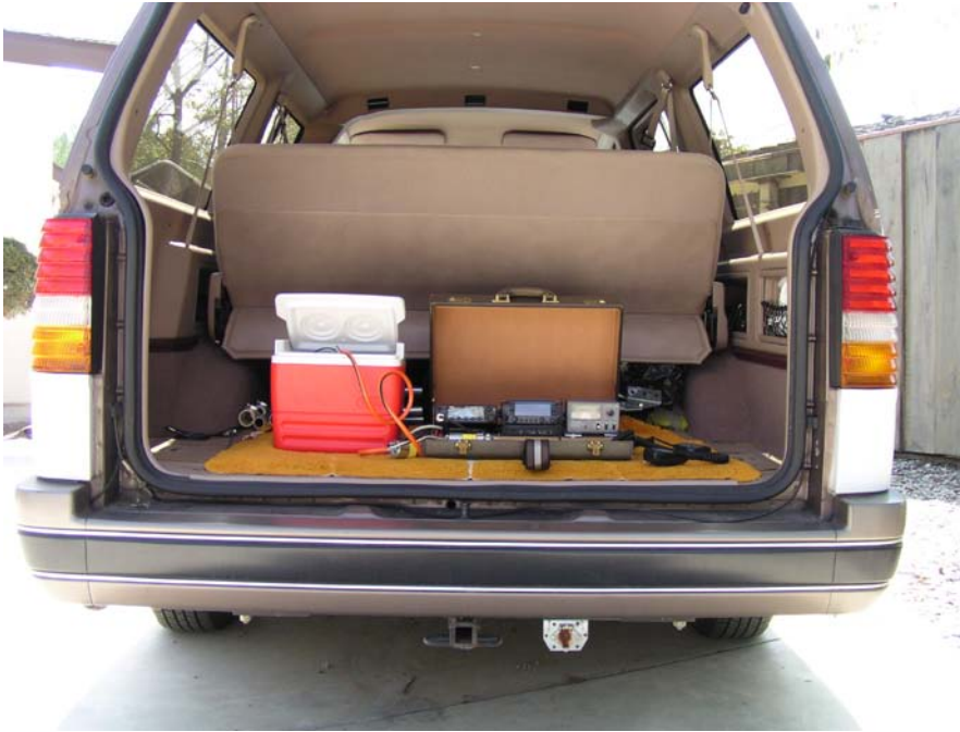
Figure 2 A Typical Cross Band Repeater Installation
